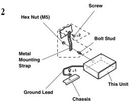
Reinforce the head unit with the metal mounting strap (not supplied). Secure the ground lead of the unit to a clean metal spot using a screw (\*1) already attached to the vehicle's chassis.
